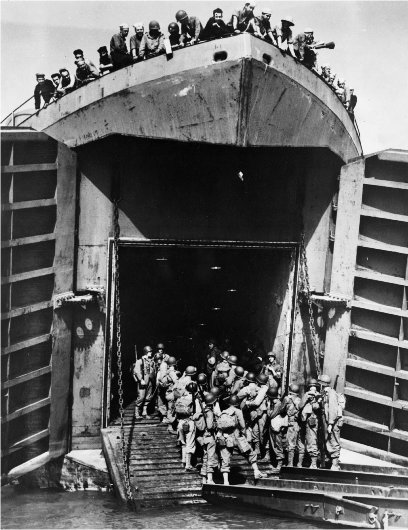
The LST could swing open her enormous bow doors to disgorge Sherman tanks directly onto a sloped beach. National Archives
