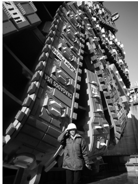
With “Big Bertha,” the gigantic machine boring the tunnel to replace the viaduct. WSDOT
